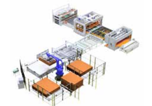
RoBOX-F Automatic Flat Mattress Boxing Robot
