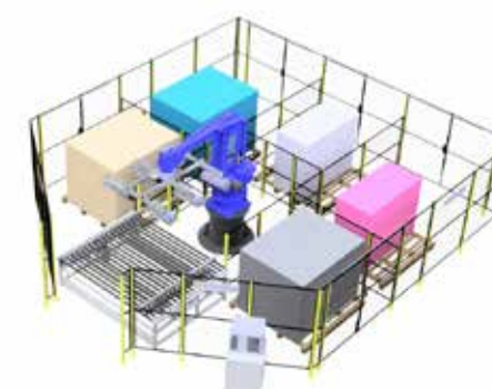
RobET-SFP Automatic Feeding and Assembly Robot
