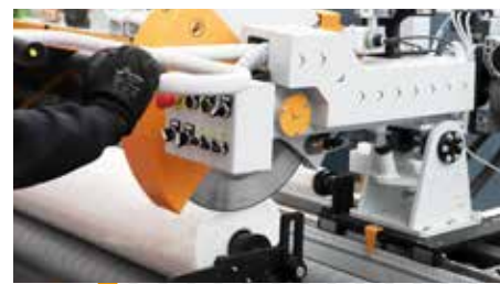
02 Motorized right and left motion of the blade
