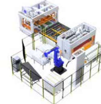
RoBOX-100 Automatic Roll Pack Mattress Boxing Robot
